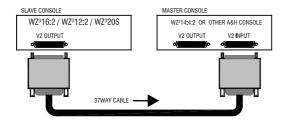
Plug the 'slave' console SYS-LINK V2 output into the 'master' console SYS-LINK V2 input. Make sure the connectors are fully plugged in and their securing screws tightened.
