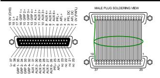
37way male to male D-type cable wired one to one. 36-core shielded cable with screen soldered to pin 19.
