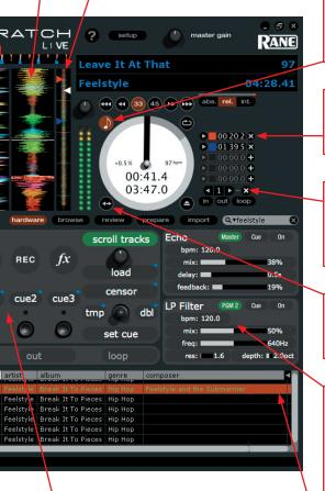
These "soft" controls have multiple functions for controlling Serato Scratch LIVE from the matched physical controls on the TTM 57SL. They also assign the Internal Digital Effects when the mixer is operated stand-alone without a computer. Six different preset groups optimize common controls for playback, cue/looping, effects, recording and library, or customize any control with a right-click. Footswitch controls are mapped here as well.
