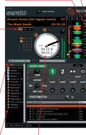
The Virtual Deck shows everything about the speed and position of a track. As the vinyl rotates, so does the line on the label. The circular progress bar around the edge is a visual representation of the position within the song. The time and remaining time are displayed in minutes and seconds. The turntable speed as a percentage of pitch shift is on the left, and the pitched BPM is on the right.
