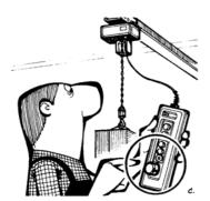
Check, when not under load, that the movement of the hook corresponds to the direction of the arrows on the control box. If not, see "Troubleshooting".
