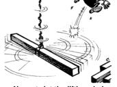
Never twist the lifting chains (turning around of the hook block)
