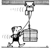
If manually moving the hoist, push the load
