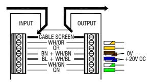
**End of chain termination** As with any RS485 system, the last **PL** device needs to have a terminating resistor fitted to its output port. Each **PL-3** is shipped with a 100 ohm resistor already fitted. Leave this fitted only if the unit is the last in the chain.
