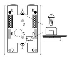
**Mounting into the face plate** A pre-cut brushed aluminium UK (part number AA5029), EU (AA5250) or US (AA5030) plate is supplied. A backing box for the UK plate can be supplied (AA5220).
