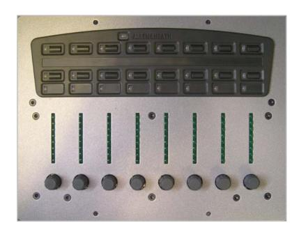
**Introduction** The **PL-10** adds to the extensive range of remote control devices available for the **iDR-4** and **iDR-8** audio mix processor systems. It offers an alternative to the **PL-6** fader controller with the advantage that user settings can be stored and recalled without the need to physically move the controls to the new settings.
