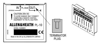
End of chain termination As with any RS485 system, the last PL device needs to have a terminating resistor fitted to its output port. The PL-10 is shipped with an RJ45 terminator plug with this resistor built in. Plug the terminator into the last unit in the PL-Anet chain. If the PL-10 is the only unit connected make sure the terminator is plugged into its output port.
