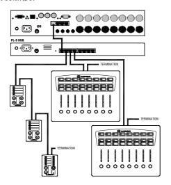
**PL-Anet** is the proprietary Allen & Heath system for daisy chaining remote controllers. It is an RS485 serial connection that uses CAT5 STP cable to communicate between devices over long distances. It requires a terminator at the last unit in the chain. PL-Anet only works with Allen & Heath **PL** devices. The connection includes +20V DC to power the connected devices. The **iDR-8** port is shown here.
