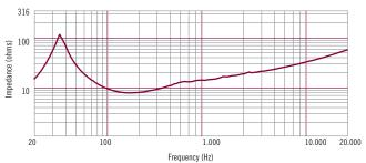
Impedance magnitude curve measured in free air.
