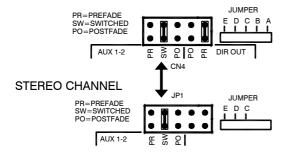
Channel Aux pre/post settings Factory default is Aux 1-4 = switched, Aux 5-8 = switched, Aux 9-10 = switched pre/post fader. You can change the setting of Aux 1-2 from switched to permanently pre-fade or post-fade if preferred. Make sure you set all mono and stereo channels the same. To avoid possible future confusion when the console is used by other operators, we recommend you only change these settings if absolutely necessary.
