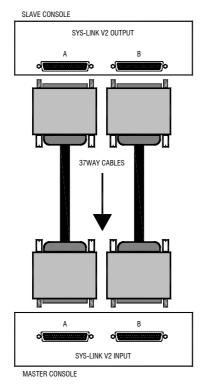
Sys-Link V2 input/output option A blank plate is fitted in both positions as standard. This may be replaced with optional cards which provide the console inputs, outputs and PFL system on pairs of 37way D connectors for linking to other Allen & Heath consoles already fitted with Sys-Link V2. The GL3800 can become an input channel expander (slave) or have its number of input channels expanded (master) when linked to other consoles.
