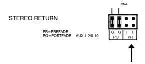
**Return Aux pre/post settings** The stereo returns feed Auxes 1, 2 and 9-10. Factory default is the post-fader so that the fader becomes a master for all feeds from the return. This may be changed to pre-fade if you prefer. Move the two jumpers from G to F.
