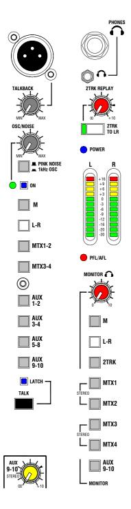
**TALKBACK** Individually assignable talkback is available to all the main outputs. Plug in a suitable cable or gooseneck microphone. A good quality dynamic or condenser vocal microphone is recommended. Note that +48V phantom power is available at the XLR as standard. If you prefer, this can be disabled by repositioning an internal jumper link.
