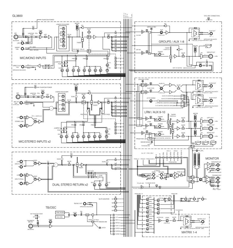
The GL3800 has a versatile architecture which should satisfy most applications you may encounter without modification. However, the following internal options provide alternative settings for those applications that may demand them. Access is required to the internal assemblies. For user convenience, pluggable jumper links are used in most places.
