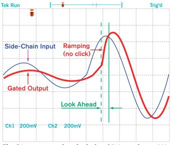
The G4 uses a very short look ahead (16 samples, or 333 microseconds) with exponential ramping to ensure accurate clickless gating.
