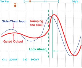
The G4 uses a very short look ahead (16 samples, or 333 microseconds) with exponential ramping to ensure accurate clickless gating.
