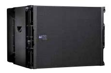
The TTL12-AS is an extremely compact high power subwoofer designed to compliment the TTL31-A Speaker System. Based around a band pass design using a newly designed 4" voice coil vented neodymium 12" woofer, it features lightweight, high force, neodymium magnet assembly, incredibly linear frequency response characteristics, the highest power handling of any comparable 12-inch transducer, the lower power compression.
