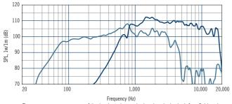
Frequency response curve of the loudspeaker make in a hemispherical, free field and mounted in a reflex box with an internal volume of 50 litres and tuned at 60Hz, applying
