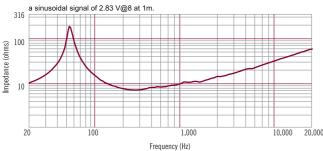
Impedance magnitude curve measured in free air.
