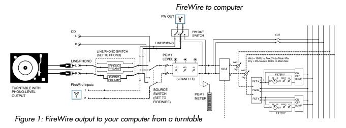
switches takes it out via FireWire to your computer. You can use the source switch to select FireWire or a CD to play into this program channel without upsetting the phono FireWire output (see dashed lines in figure 1). This would be the way to play a timecode record. While on the subject, I feel a paragraph or two coming on...
