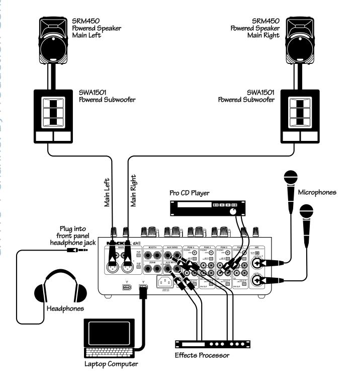
This diagram shows a CD player and microphones connected, with an effects device in the aux loop, and a laptop attached. Various popular DJ software such as Traktor™, PCDJ™, and MixVibes™, can be used with the d.4 Pro via the FireWire connection. The main mix can also be recorded with software such as Tracktion.
