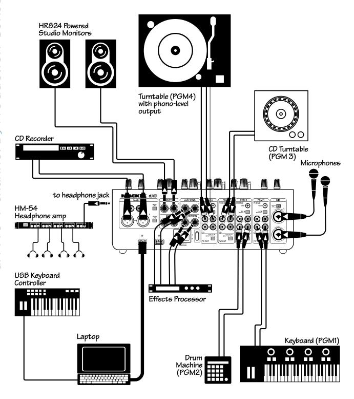
This diagram shows a keyboard, drum machine, turntable and CD turntable, with two microphones. A USB keyboard controller is also attached directly to the computer. The FireWire output from various software, such as Reason<sup>TM</sup>, Abelton Live<sup>TM</sup>, Tracktor<sup>TM</sup>, Tracktion<sup>TM</sup>, and Logic<sup>TM</sup> can be sent to the four program channels for mixing. An effects processor is also shown in the aux loop.
