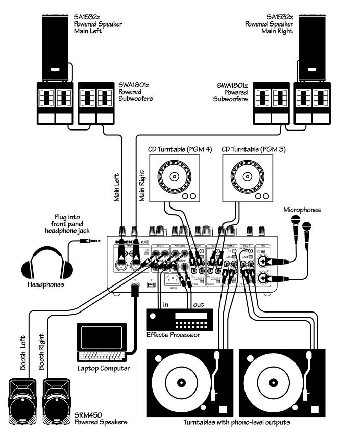
This diagram shows 4 sources hooked up to 4 channels, with an effects device in the aux loop, and a laptop attached. Separate tracks can be recorded into Tracktion, of each stereo program channel and the microphones, and even the effects channel. This gives multitrack recording of all the elements of the performance, for remixing at a later time.
