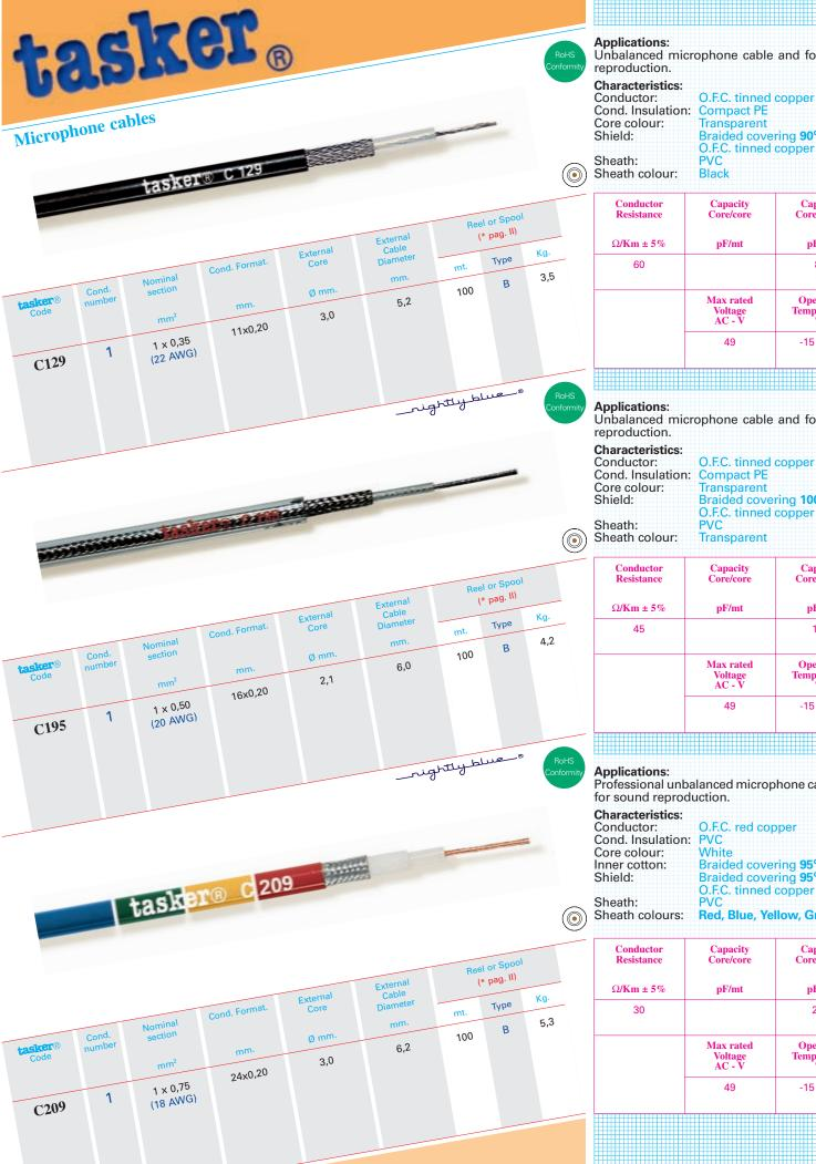
Unbalanced microphone cable and for sound
