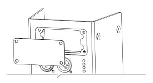
2 - Connect the flat cable that you find inside the speaker to the RDNet plug accessory
