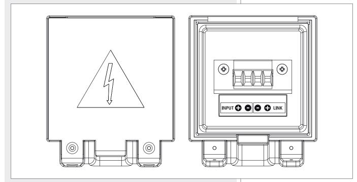
The two INPUT contacts (+ and -) allow the connection of the input cable, the two LINK contacts (+ and -) can be linked to an output cable for the parallel connection of other speakers.
