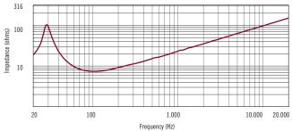
Impedance magnitude curve measured in free air.
