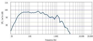
Frequency response curve of the loudspeaker make in a hemispherical, free field and mounted in a reflex box with an internal volume of 250 litres and tuned at 40Hz, applying a sinusoidal signal of 2.83 V @8 at 1m.
