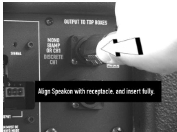
To connect a Speakon, insert the keyed plug into the receptacle and twist counterclockwise to lock in place.
