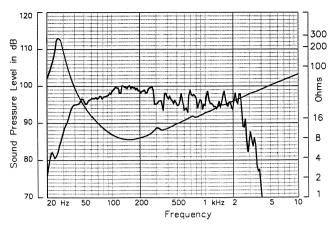
Response measured in a half space environment using a vented enclosure of 208 litres.
