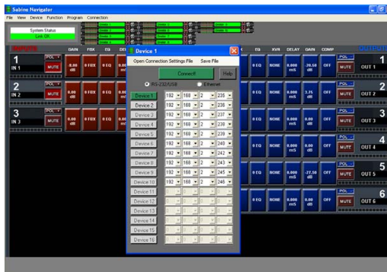
Main screen in Navigator Software, showing Connection window with IP addresses assigned and 10 devices present. Note System Status at upper left shows the units are already connected.
