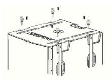
Each product also includes four (4) M10 threaded Permanent Installation (PI) suspension points on enclosure top and bottom. The figure to the left illustrates their locations in the NTS250 top panel. M10 forged shoulder eyebolts or similar load-rated hardware may be used in these points when deploying NTS250 subwoofers in permanent installation applications.
