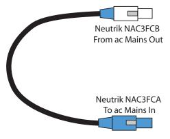
Recommended cable length for connecting vertically adjacent enclosures = 300 mm to 450 mm / 12 in to 18 in
