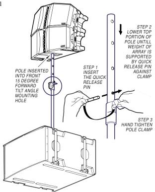
**CAUTION:** All enclosures must be securely pinned together. Be sure that the subwoofers are stabilized and secured from falling over or being accidentally pushed over.
