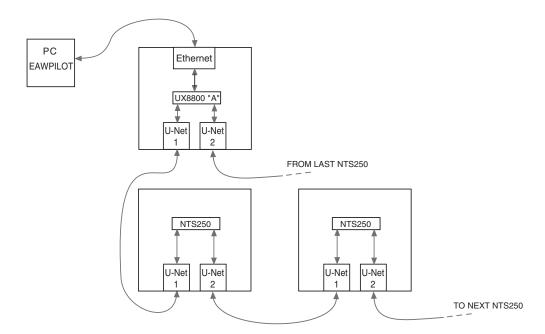
It is recommended that you connect the first free U-Net port to the first NTS250. A ring is created so the audio and control signals have two paths along the network, and the integrity of the network is maintained in the event that one NTS250 should go offline.
