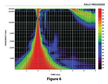
To solve this dilemma, the company undertook development of custom (and rather radical) DSP algorithms specifically engineered to provide the required filters for correcting loudspeaker anomalies. The resulting filters had to possess the required precision and accuracy in both the frequency and time domain. At the same time, any uncorrectable anomalies would have to be ignored by the filters.
