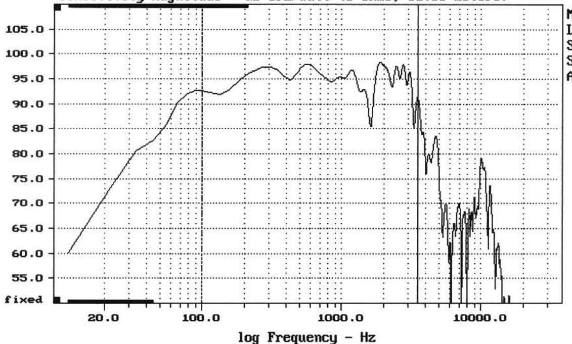
**Level (100:3507 Hz) = 95.48 dB SPL/watt (8 ohms, @1.50 meters)**
