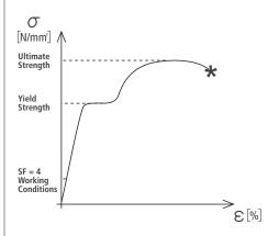
The safety factor is the result of the forces acting on fly bar's and system's front and rear links and pins and depends on many variables:
