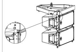
4) Reverse and connect the 2 rear bracket to the fly-bar using 2 quick lock pins. The first HDL20-A has to be fixed always starting at 0° with respect of the frame. No other angles are allowded.
