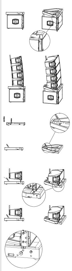
4) The baffle of the bottom box in a stacked array does not necessarily have to be parallel to the stage or the array frame. It can be tilted up or downward if desired. In this way arced arrays can be readily created from a ground stack position.
