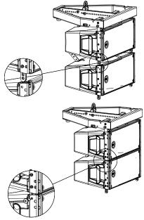
6) Reverse and connect the rear bracket of the second cabinet using the hole for the proper angle.
