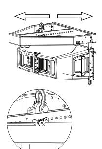
8 Check that all the pins are secured and locked.
