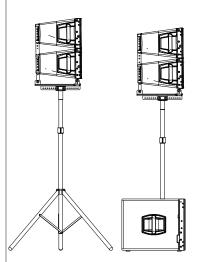
**WARNING**: The floor stand support the full load of the part of the system on top. It is very important that the floor stand is certified for the total weight on top.
