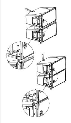
3) Reverse and connect the rear brackets of the first cabinet using the hole for the proper angle.
