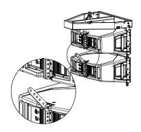
7) Connect all the other cabinets following the same procedure and connecting a single cabinet each time.
