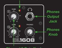
Channel 8 Gain Knob Figure B – Front Panel
