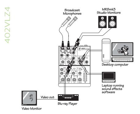
This diagram shows two voice-over microphones connected to the mic inputs of channels 1 and 2.
