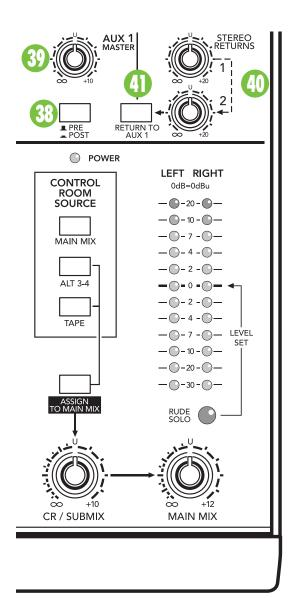
These outputs can be fed to the inputs of a reverb or other device. From there, the outputs of this external device are fed back to the mixer's stereo return [7] jacks. then these signals are sent through the stereo return [40] level controls, and finally delivered to the main mix.
