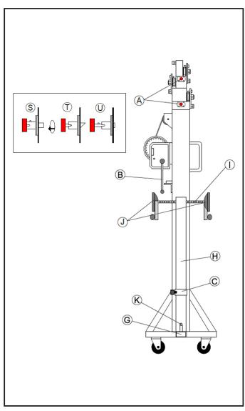
the profiles with the safety pins (A) in the position (S).
