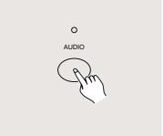
5. To return to normal mode, tap the Audio button a second time causing its LED goes out, the Audio mode is disengaged.
