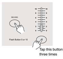
2. Tap the Flash button 5 or 10 three times while holding down the Record button.
