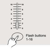
2. Tap the Flash button numbered from 1-16 to assign MIDI OUT channel 1-16, the relevant channel LED lights indicating MIDI OUT channel is set.
