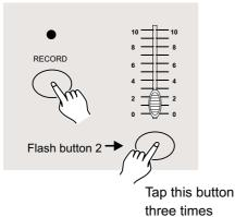
Tap the Flash button 2 three times while holding down the Record button, the Segment Display reads "CHO" indicating MIDI OUT channel setup is available.
