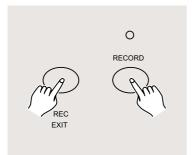
5. Tap the Rec Exit button while pressing and holding down the Record button, the Scene LED goes out, indicating the exit of Edit mode.
