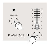
7. Press a Flash button between 13-24 while holding down the Record button. All LED will flash indicating the scenes have been programmed into memory.
