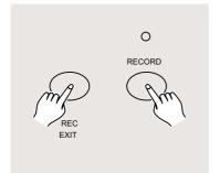
Press and hold down the Record button. While holding down the Record button tap the Rec Exit button to exit MIDI setting.
