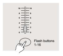
2. Tap the Flash button numbered from 1-16 to assign MIDI IN channel 1-16, the relevant channel LED lights indicating MIDI IN channel is set.
