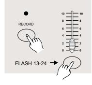
Press a Flash button between 13-24 while holding down the Record button. All LED will flash indicating the scenes have been programmed into memory.
