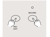
You can continue programming or exit. To exit Program mode, tap the Exit button while holding down the Record button, the Record LED should go out.
