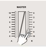
3. Push Master Slider B to its maximum position(fully down).
