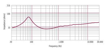
Impedance magnitude curve measured in free air.
