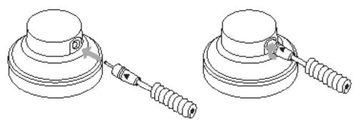
In order to lock your selected cable into the Pro Set 3 you simply insert and twist to lock.
