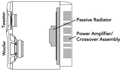
Figure 1. HR624 MK2 Cutaway side view
