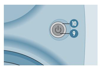
When the POWER MODE [6] switch is in the ON position (and the front panel power switch [9] is in the IN position), applying AC power activates the muting circuit for about four seconds while the power supply and internal circuitry stabilize, then the HR624 MK2 unmutes and is ready to go.
