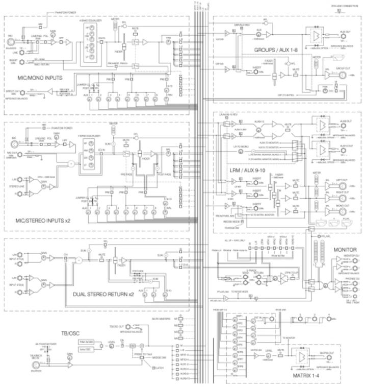
GL3800 System Block Diagram
