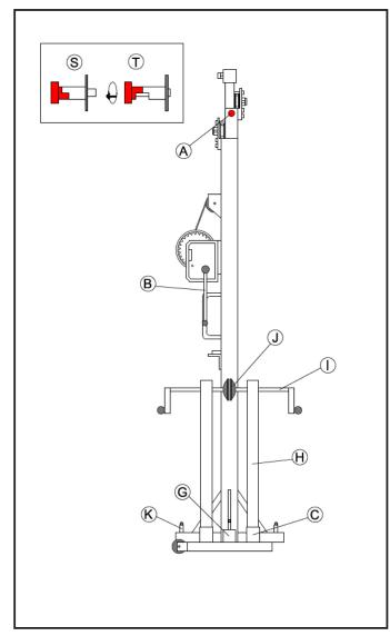
the profiles with the sa ety pins (A) in the position (S).
