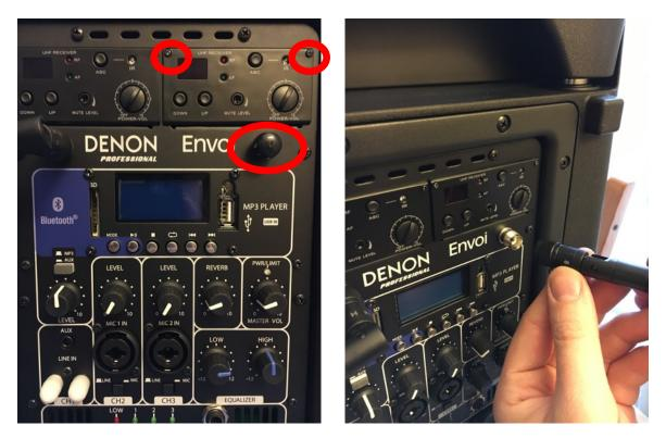
Switch on the receiver and select a different channel to the one selected on the first receiver.
