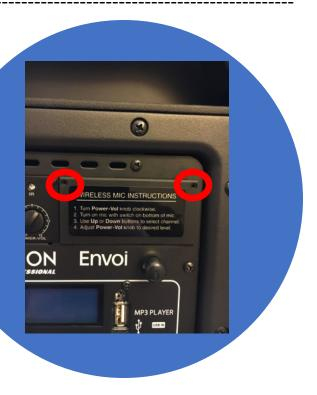
Remove the two screws as highlighted
