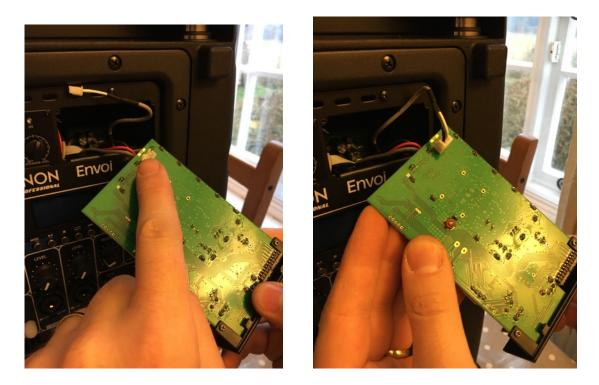
Now slot the receiver in to the Envoi taking care not to trap the cables.
