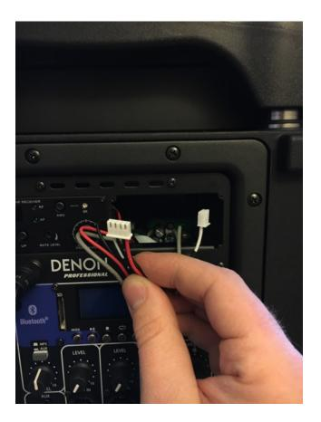
Plug the large connector to the socket on the top side of the board
