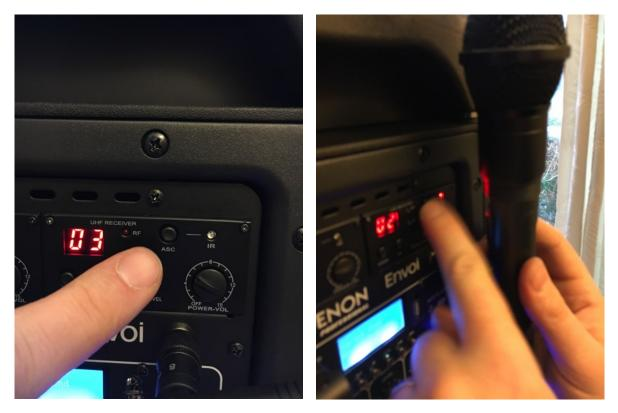
Point the microphones IR receiver towards the LED. When connected the "RF" LED will light up.
