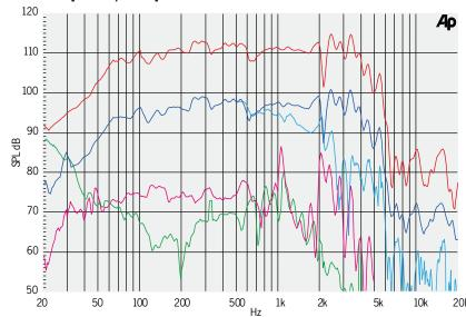
Data measured using swept sine wave input on an open baffle of dimensions  $2.5 \times 3.7$  metres with a microphone distance of 1 metre.
