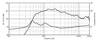
Frequency response curve of the driver measured on-axis at a distance of 1 meter with a 1 watt input signal in an anechoic environment mounted on a horn with a Q of IS.
