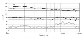
Measurements made at 1 meter distance with an input signal whose power is equal to 10% of the driver's rated power mounted on a horn with a Q of IX
