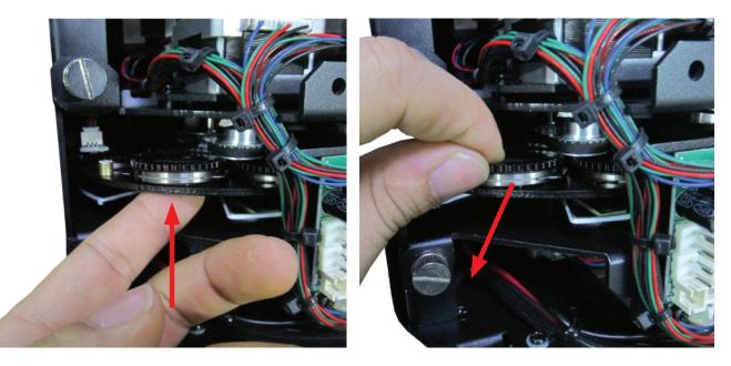
4. Place the gobo holder with the black gear side down. Using a set of tweezers, remove the retaining spring by grasping the end of the spring with the bent tip (right).
