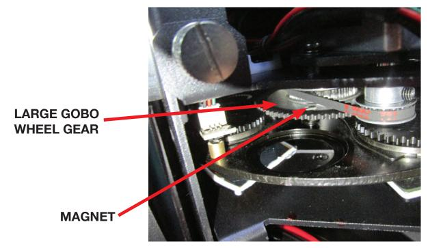
9. Making sure that the mark on the geared portion of the gobo holder is still aligned with the gobo holder clip, insert the clip of the gobo holder onto the attachment point on the gobo wheel. You should hear an audible click as the gobo holder snaps into place.
