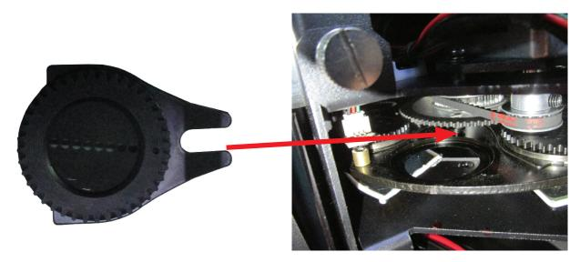
10. Gently push the gobo holder upwards from below, until the silver portion of the gobo holder clears the surface of the gobo wheel. Hold the gobo holder in this position and rotate the gobo holder so that the mark on the black geared portion is aligned with the small circular magnet on the large gobo wheel gear.
