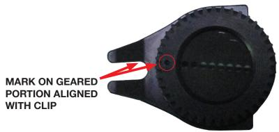
8. Locate the large gear on the gobo wheel that meshes with the geared parts of the gobo holders. Rotate the gobo wheel to turn this large gear until the small, circular magnet on this large gear in pointing outwards.
