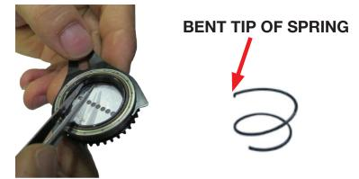
5. Remove both the retaining spring and the gobo from the gobo holder.
