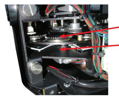
Gobo being changed is aligned to open slot in color wheel
