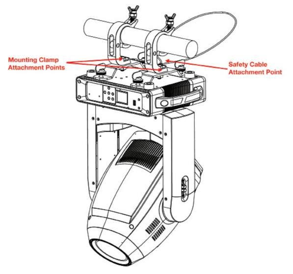
When installing the unit, the trussing or area of installation must be able to hold 10 times the weight of the unit and any attached accessories without any deformation. The unit must be secured with a secondary safety attachment, e.g. an appropriately-rated safety cable. Never stand directly below the unit when mounting, removing, or servicing the unit.
