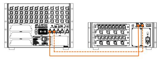
Switch on the MixRack first, then the DX Expander. The DX port Lnk/Err indicators flash at a steady rate when the link is established. The red error indicator lights if a communication error is detected. Check that the cables are correctly plugged in and are not faulty.
