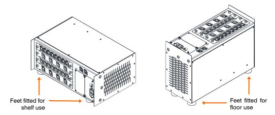
(i) Ensure adequate air flow around the unit. It must not be covered in any way. Always stand the unit on a firm flat surface away from any soft furnishings or carpet.
