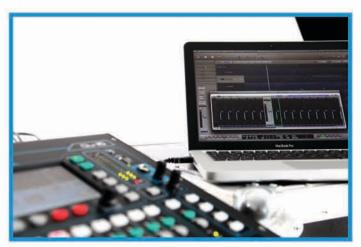
The returns from the Mac can be assigned to the Input channels. The interface is class-compliant on Mac OS X – which means it's truly plug 'n play, with no need to install a driver. It will be recognized straightaway by any DAW supporting Core Audio, including Logic, Cubase, Reaper, and Pro Tools.
