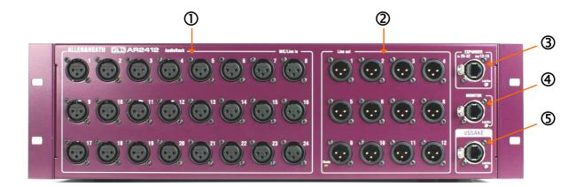
Input sockets 24 balanced XLR inputs for microphone and line level sources. The preamps are built into the AR2412 rack and their Gain, Pad and 48V phantom power is remote controlled from the GLD console via the dSNAKE link. The output of the analogue preamps are converted to digital format and transported via dSNAKE to be processed and mixed at the GLD-80 mixer.
