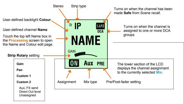
Select the function of the strip Rotary controls using these keys. The Custom keys are assigned using the Setup / Control / Surface Prefs screen.
