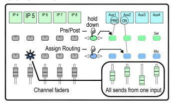
Press an Input Channel strip Mix key.
