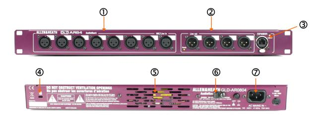
Input sockets 8 balanced XLR inputs for microphone and line level sources. The preamps are built into the AR84 rack and their Gain, Pad and 48V phantom power is remote controlled from the GLD console via the EXPANDER link. The output of the analogue preamps are converted to digital format and transported via a Cat5 cable to be processed and mixed at the GLD-80 mixer.
