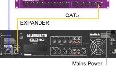
Connect the AR2412 AudioRack Plug a CAT5 cable into the dSNAKE port at the rack and mixer. This is the main system link.
