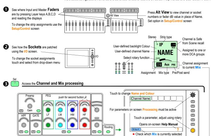
For GEQ on faders press GEQ Fader Flip - Master on last fader. RTA on strip meters. RTA follows current selected PAFL
