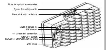
Notes: For mounting, a variety of accessories can be attached using the 3/8" thread on the backside of the LED Panel (see "Grip accessories" on page 19).
